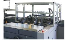
While it lacks cardboard during conveying, there is an auto detector.(The machine will stop can alarm while lacking one or several pieces of cardboards in conveying)
