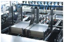
While it lacks cardboard during conveying, there is an auto detector.(The machine will stop can alarm while lacking one or several pieces of cardboards in conveying)
