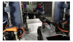
◆ Adopt new design of servo and pneumatic control structure to wrap the box, fast digital adjustment of sizes.
