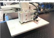
• Box pre-press device, fix the paper and box tightly and remove the bubbles.
