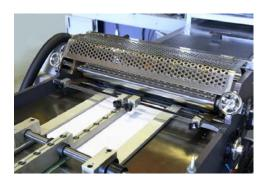
◆ Gluing cylinder is made of finely-grinded and chromium-plated stainless steel. It is equipped with line-touched type copper doctors, more durable.
